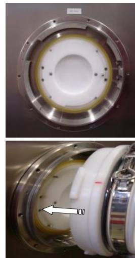
Abb.: RTP Rapid Transfer Port
